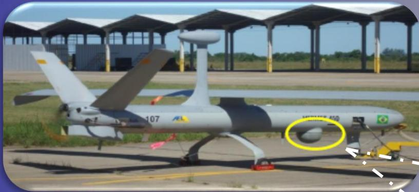
Digital Compact Multi-Purpose Advanced Stabilized System (DCoMPASS)
